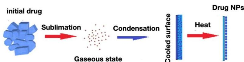
*Fig. 1. Scheme of the experiment on cryogenic production of nanoparticles*
